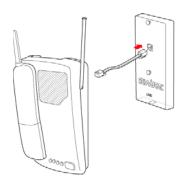
4. Attach the telephone to the mounting pegs on the DSL filter and your installation is complete.
